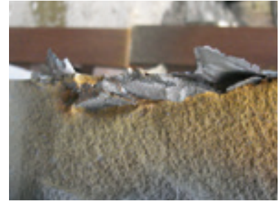
Appearance of drawing-step overlaps at the end of a bar.
