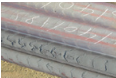
Drawing-step overlaps on a rectangular bar as cast.
