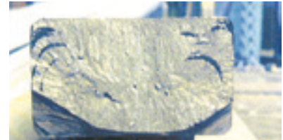
Fracture surface displaying chill.
