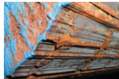
Scores on a large diameter round bar.
