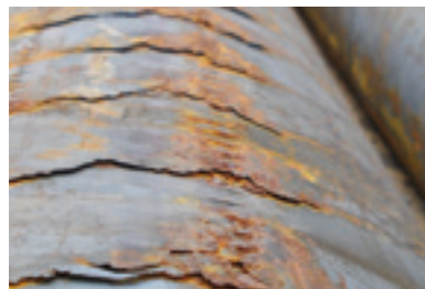
Drawing-step overlaps on a round bar as cast.
