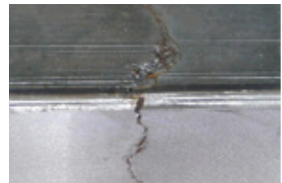
Drawing-step overlap on a rectangular bar machined on one face.
