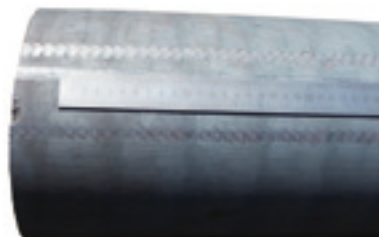
Longitudinal marks derived from the pulling device.
